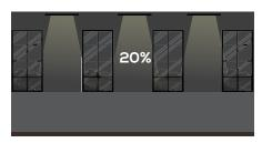
After an additional 3 minutes elapse the sensor dims the light to 20% light level.
